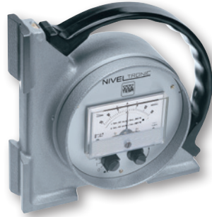
NIVELTRONIC square model with 2 prismatic bases
