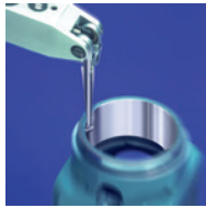
GT 31 with lever in perpendicular position
