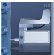
Perpendicularity using TESA IG-13
