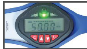
The green LED illuminates within 4% of target torque. Continuous buzzer sounds when target is reached.
