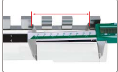
check upper jaws of caliper
