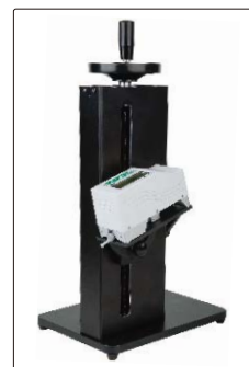
light duty test stand (optional)
