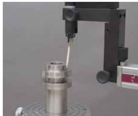
Spiral-mode cylinder measurement
